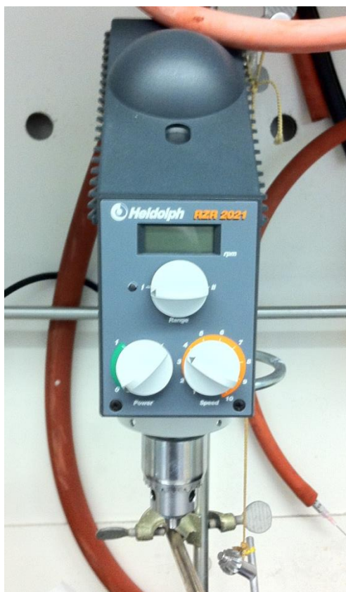
FIGURE 2—Heidolph overhead stirrer used for mechanical mixing of solutions.
