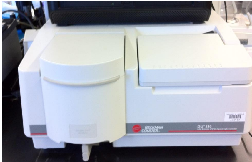
FIGURE 3—Spectrophotometer used for absorbance measurements.
