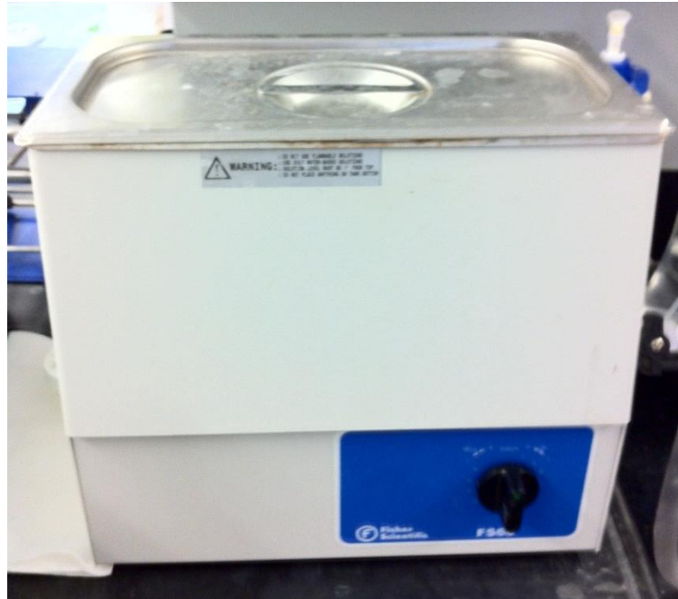
FIGURE 1—Ultrasonic Cleaner used to indirectly mix solutions
